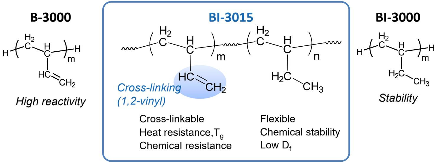
BI-3015 is partial hydrogenated Polybutadiene (85% of Butadiene units) which is derived from B-3000.
