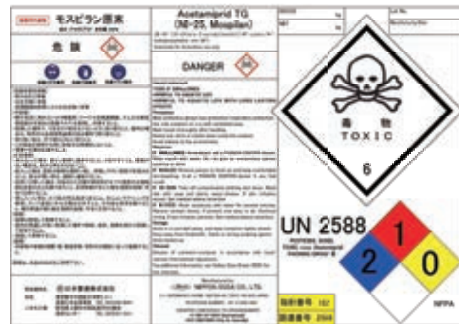
Example of a combined label The guide number and the United Nations number are printed at the bottom of the Container Yellow Card.
