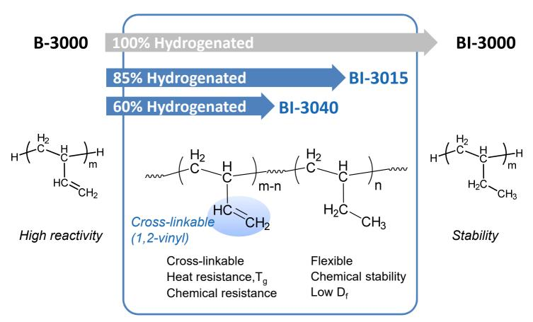
BI-3015 and BI-3040 are partial hydrogenated Polybutadiene which is derived from B-3000.
